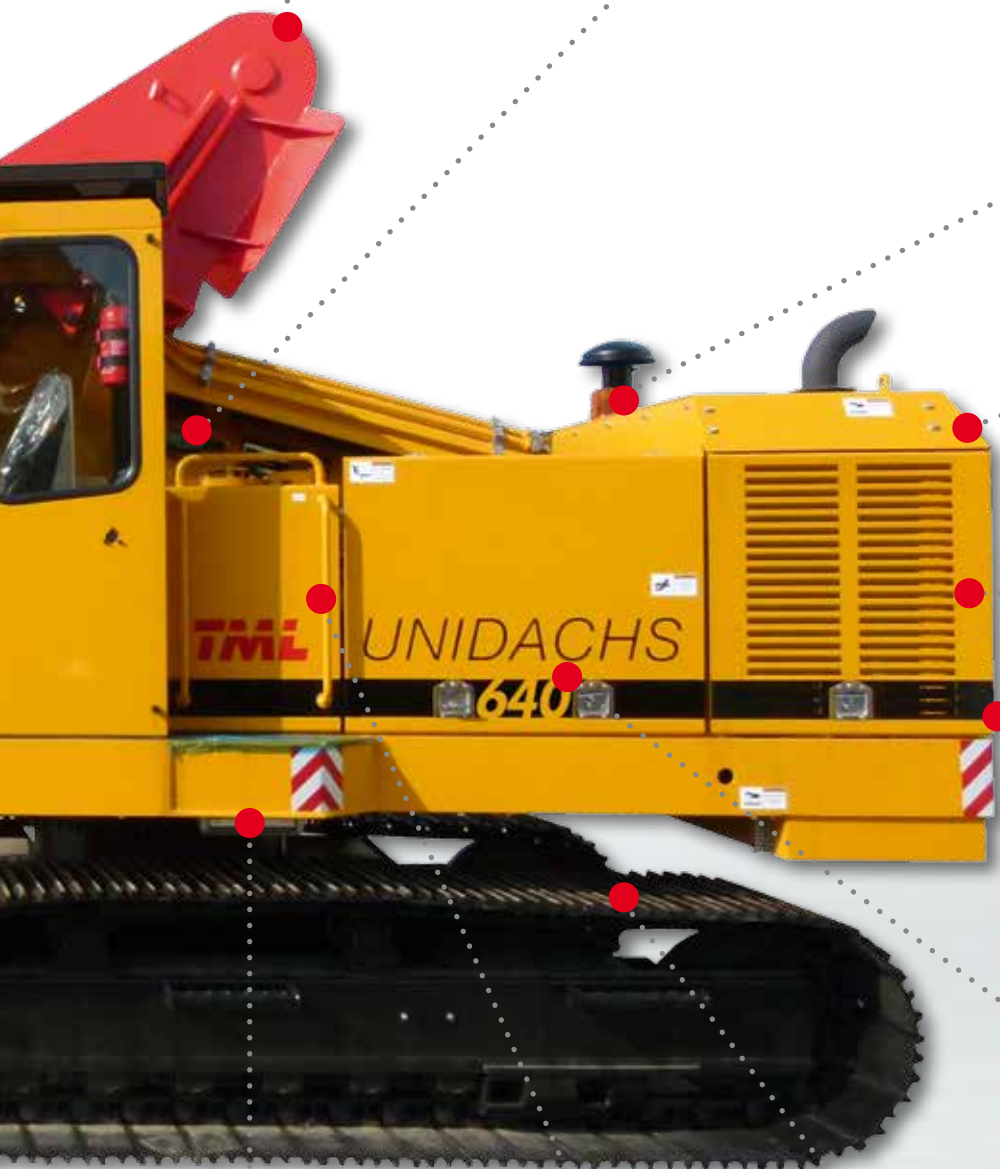
Handrails and steps for safe access to the machine super- structure and for re-fuelling
